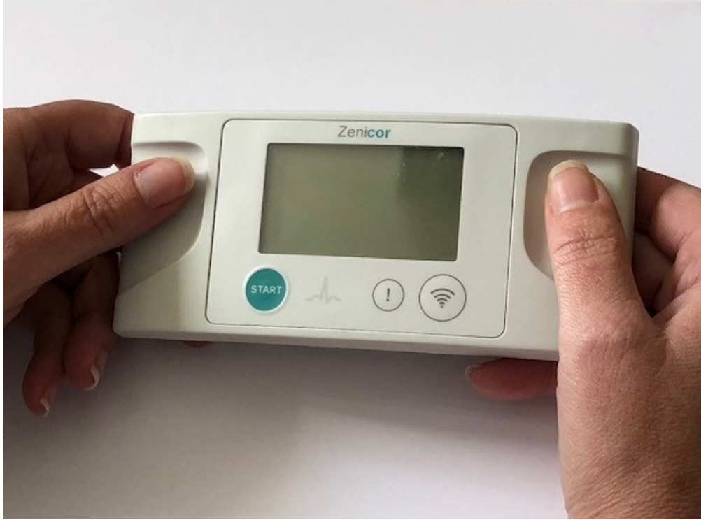
Figure 2. Zenicor hand-held ECG device used to screen for AF in the SAFER trial
